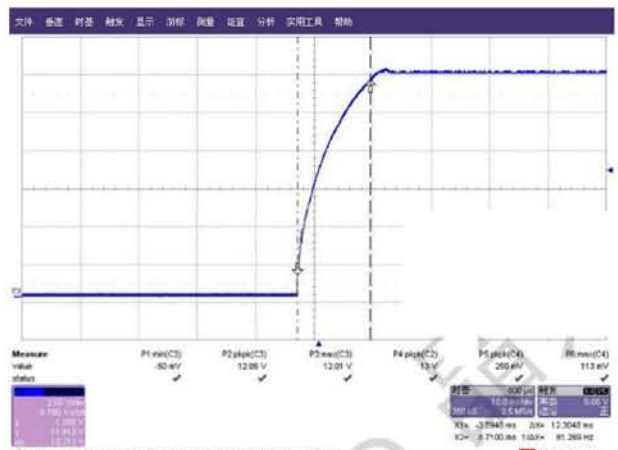
Figure 12: Rise time measured waveform@100Vac/60HZ,full load
