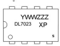
X: A for DIP8 C for SOP8
